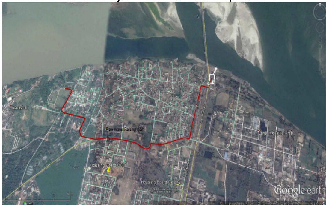
Figure 3: Google Earth map depicting proposed alignment of raw water rising mains from jackwell to water treatment plant
