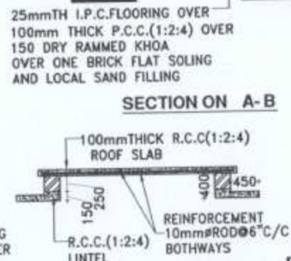
DETS OF ROOF SLAB
