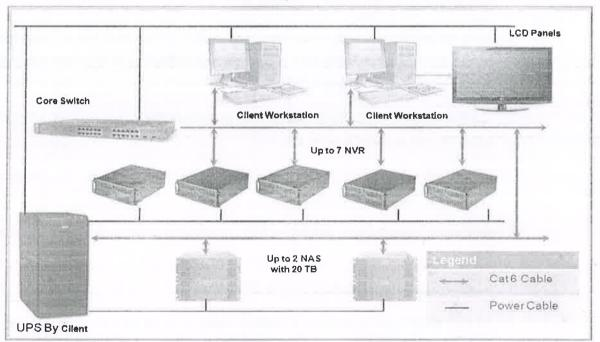
The main servers and video management application will be placed atMain Control Room with a Core Switch connecting the main camera Network from sub-Control room to the Main server at Central Control Room. The Monitoring stations are connected to the network via switch and will be places at various stated viewing locations across the cities. The Viewing station will be directly/indirectly connected to the main server for retrieving the recording or viewing the live video.
